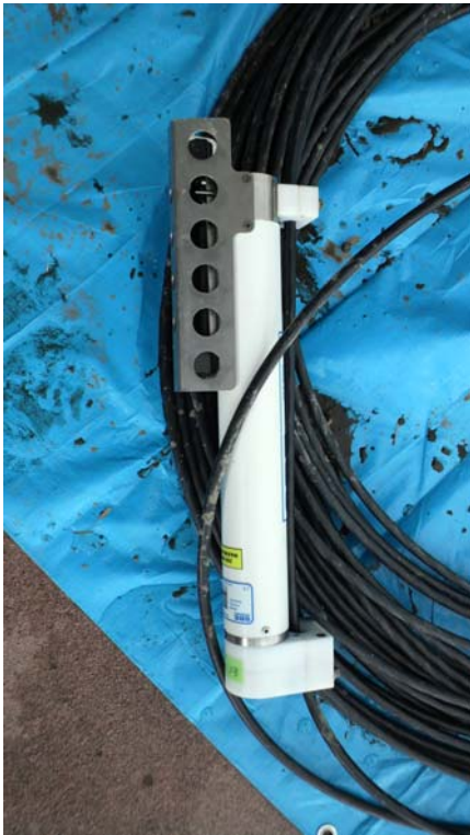
Fig. 3 Temp and conductivity sensor unit attached on the stainless wire.
